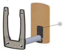
**A:** Lay the over bed table on its end or side. Take a #2 Philips screwdriver and remove the six screws that attached the table top to the column.
