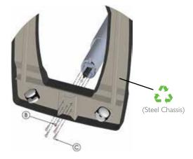
**B & C:** Using a M10 socket and ratchet, remove the M10 nut which secures the gas spring to the base. Next, using a 5/16 Allen key detach the base from the column.
