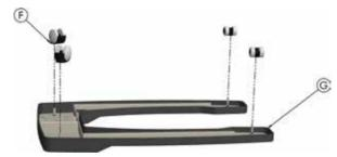
**F & G:** Lay the over bed table base upside down on a table and remove the casters by prying them upward with a large flat blade screwdriver. A small black of wood under the screwdriver shaft will provide more leverage. Next take the screwdriver and pry the ABS plastic cover off of the metal base chassis.
