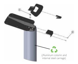
**D & E:** Next step is to remove the gas spring from the top end of the column. First, using an 8/32" Allen key, remove the Paddle retainer and lift off the paddle.
